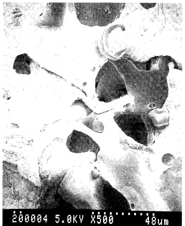
Fig. 5 Photograph of thermal spray self-bonding aluminum bronze copper aluminum coating. Top view of surface: 500\times —0.48- \mu\text{m} legend length.
